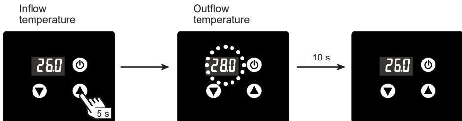
Then adjust the by-pass to obtain a difference of 2°C between the inflow and the outflow.
