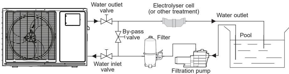
Note: The swimming pool heat pump unit is sold without any treatment or filtration equipment. The components shown on the diagram are parts to be supplied by the installation engineer.
