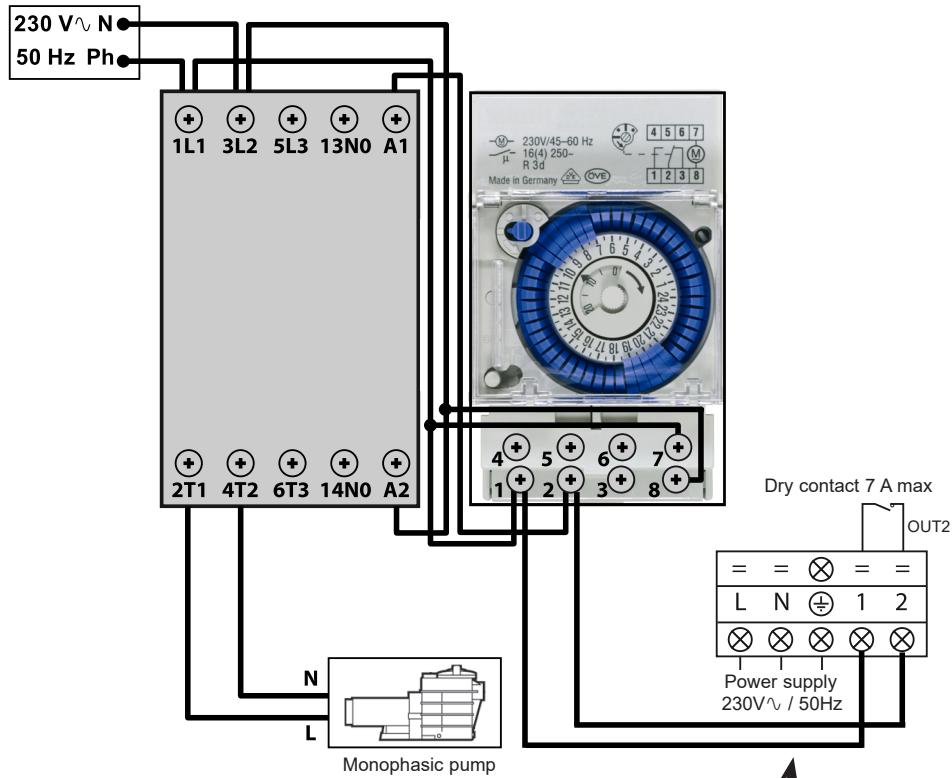
Terminals 1 and 2 deliver a potential-free dry contact, 230 V~ / 50 Hz, no polarity.
