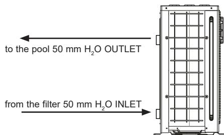
Install by-pass valve between the inlet and outlet on the heat pump.
