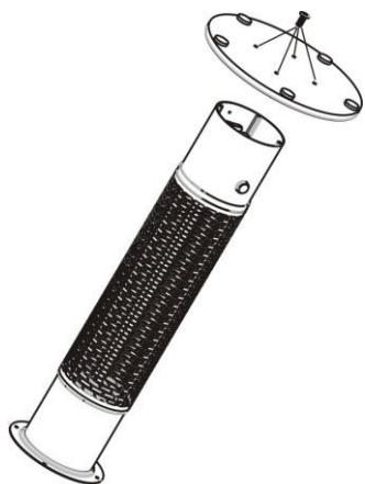
Step 2: Fix heater body with glass by 4pcs M5\*14mm screws
