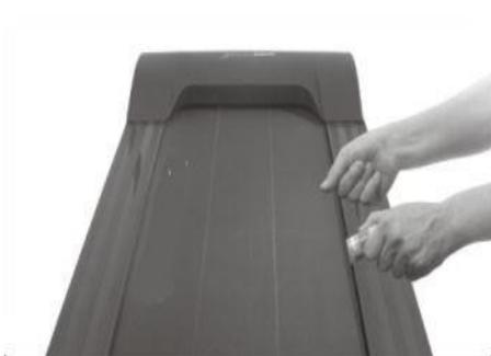
Pull up tightly of the running belt. Then put the silicone oil to running board. Then start the machine to running 3 minutes without loading. It is better to maintain like this every 30 hours working of the machine. This can save lifetime of parts properly.
