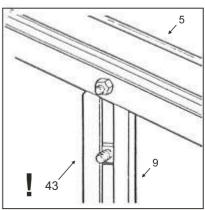
Used to show the assembly of pole 21#63#:insert a screw 43# into the pole 8#&9# before assembly(pic [B])
