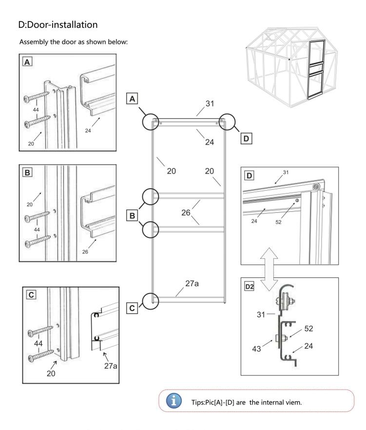
For the planar view of the assembly of the door.
