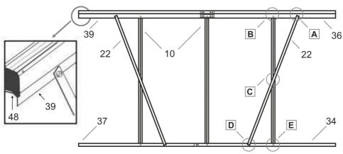
Used to show the assembly of pole 22#:for the 1st,3rd pole 10#,insert the screw 43#(pic [B]&[C])
