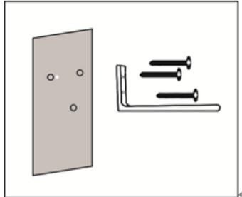
IV.Before fixed the heater,make sure the rocker power switch on the right side and then fixed the bracket and heater by two M6\*14 screws and butterfly nuts.
