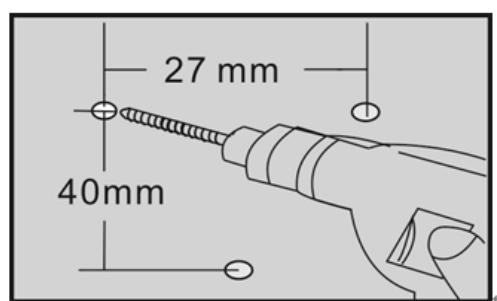
II.Insert the three plastic wall anchors to the three holes
